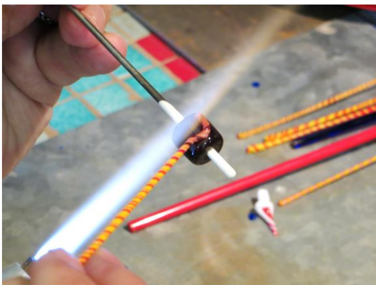
A replica Anglo-Saxon bead being made with a modern mandrel and blowtorch by Mike Poole of Tillerman Beads.
